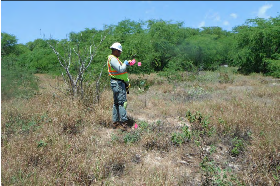
Photograph 1: Field personnel using GPS unit to locate incremental sample (IS) location at DU9, facing west.
