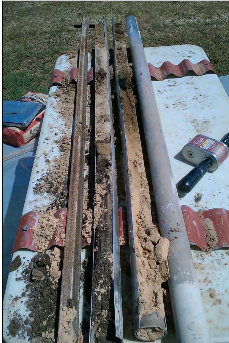
Photograph 5. Soil from SB04. Liner on the left shows soil from 0' to 5' bgs; liner on the right from 5' to 10' bgs. Shallow layer of silty brown soil observed and sampled from 1.8' to 2.4' bgs. Second layer of brown soil observed from approximately 3.5' to 6' bgs.
