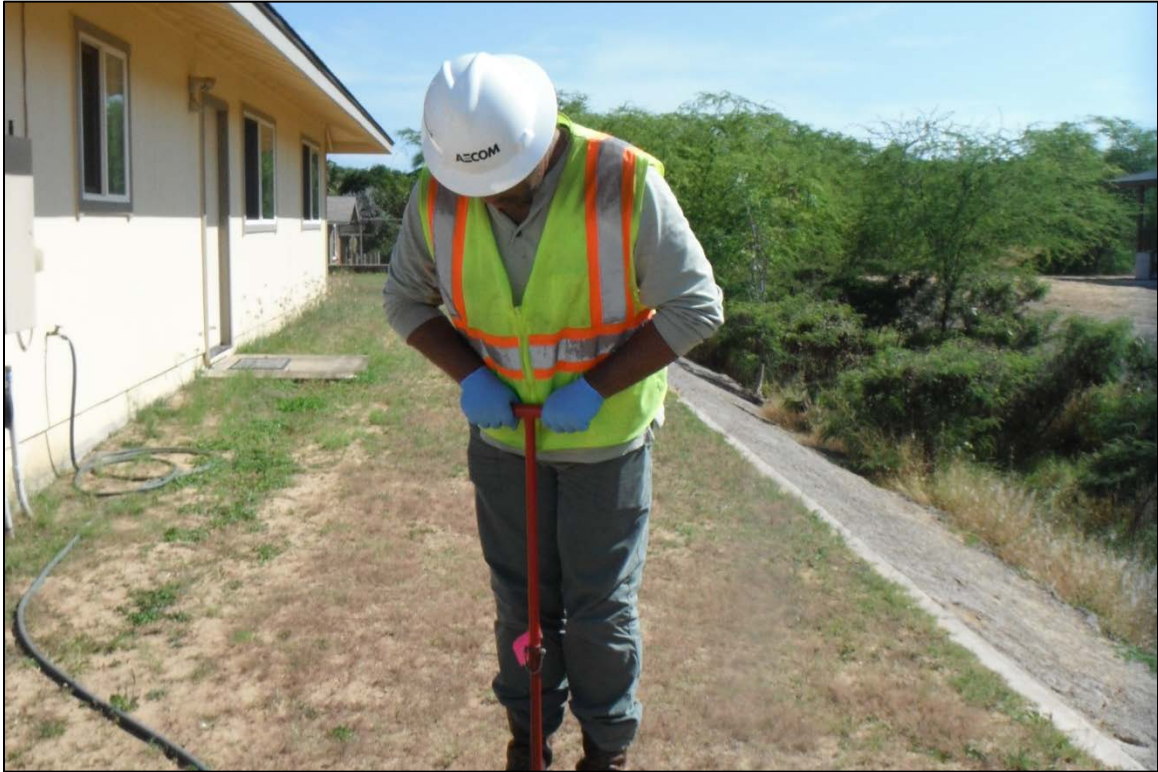
Photograph 8: Field personnel using the Cold Regions Research and Engineering Laboratory Multi-Increment Sampling Tool (CMIST) sampling tool for surface soil increment collection.
