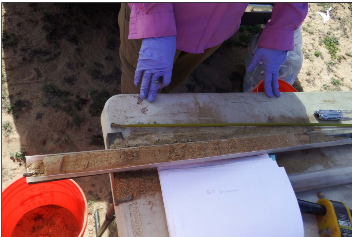
Photograph 27: Boring B-02 Duplicate Increment in Lot 51 (May 13, 2015). Typical photograph to illustrate boreholes with Layer A only (no Layer B present).
