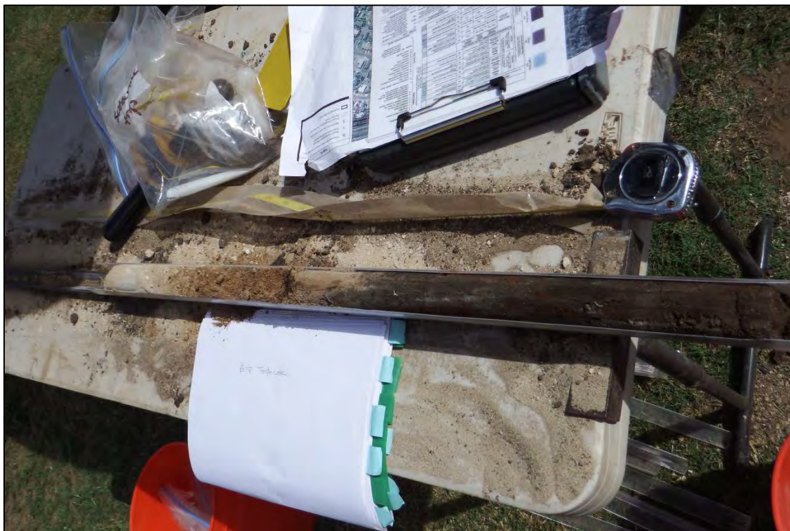
Photograph 26: Boring B-19 Triplicate Increment in Lot 15/& 16 (May 12, 2015). Typical photograph to illustrate thick (>3 inches) of Layer B, which is buried >12 inches bgs.
