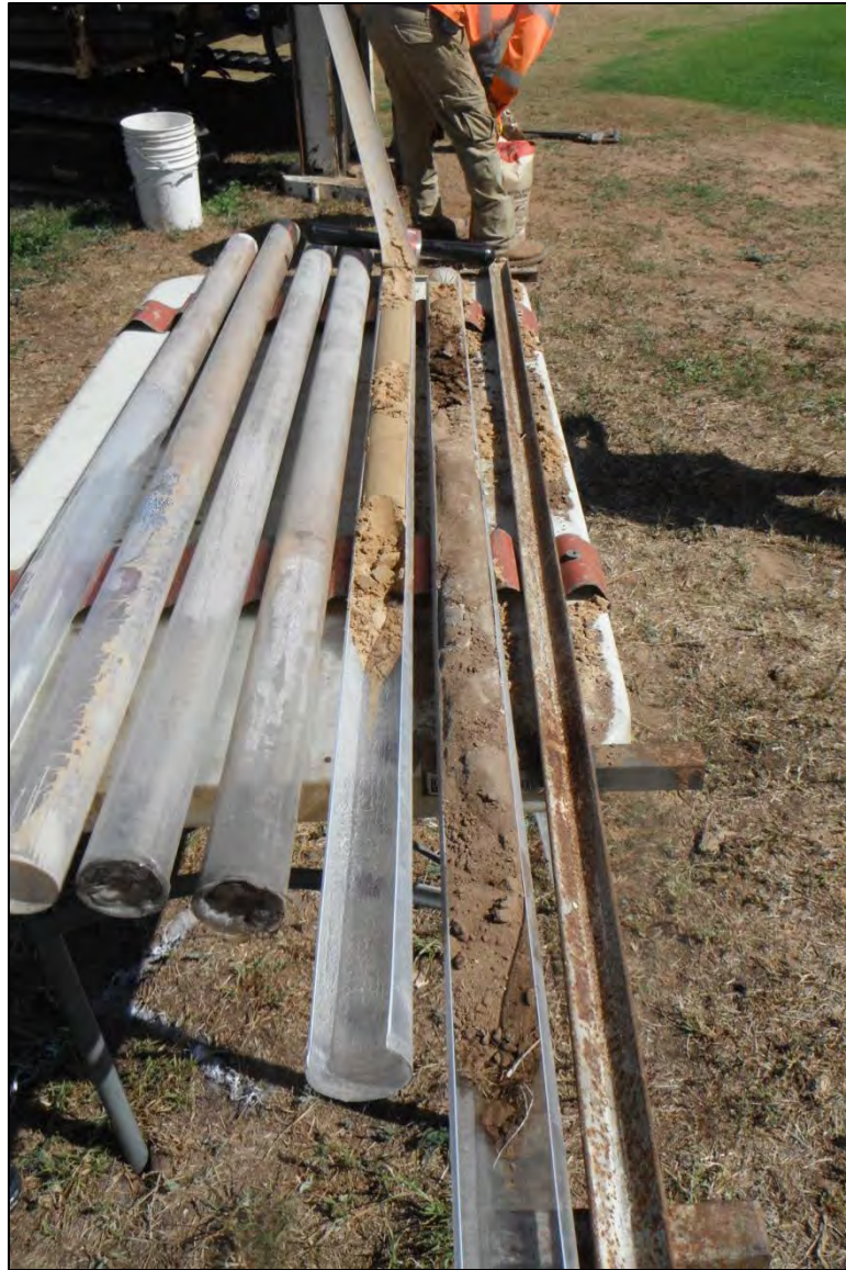
Photograph 3. Soil borings from SB02. Soil in liner on the right is from 0' to 5' bgs. Distinct dark brown silty sand layer present from approximately 3.7' to 4.4' bgs. Soil in liner on the left is from 5' to 10' bgs. No brown layer present, only native tan fine-grained sand.
