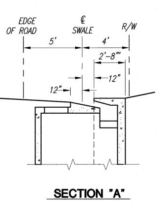
LIMIT OF EXCAVATION FILL VOID W/CONTROLLED LOW STRENGTH MATERIAL (CLSM)
