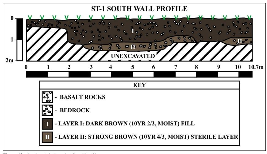
Figure 12: Stratigraphic Trench 1 South Profile.
