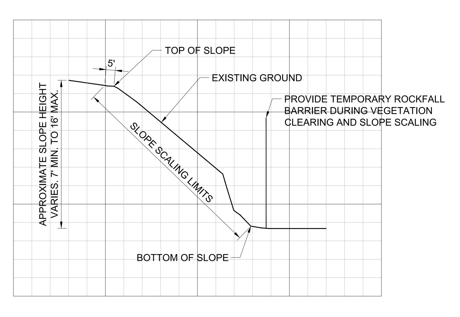
TYPICAL SLOPE SCALING NOT TO SCALE
