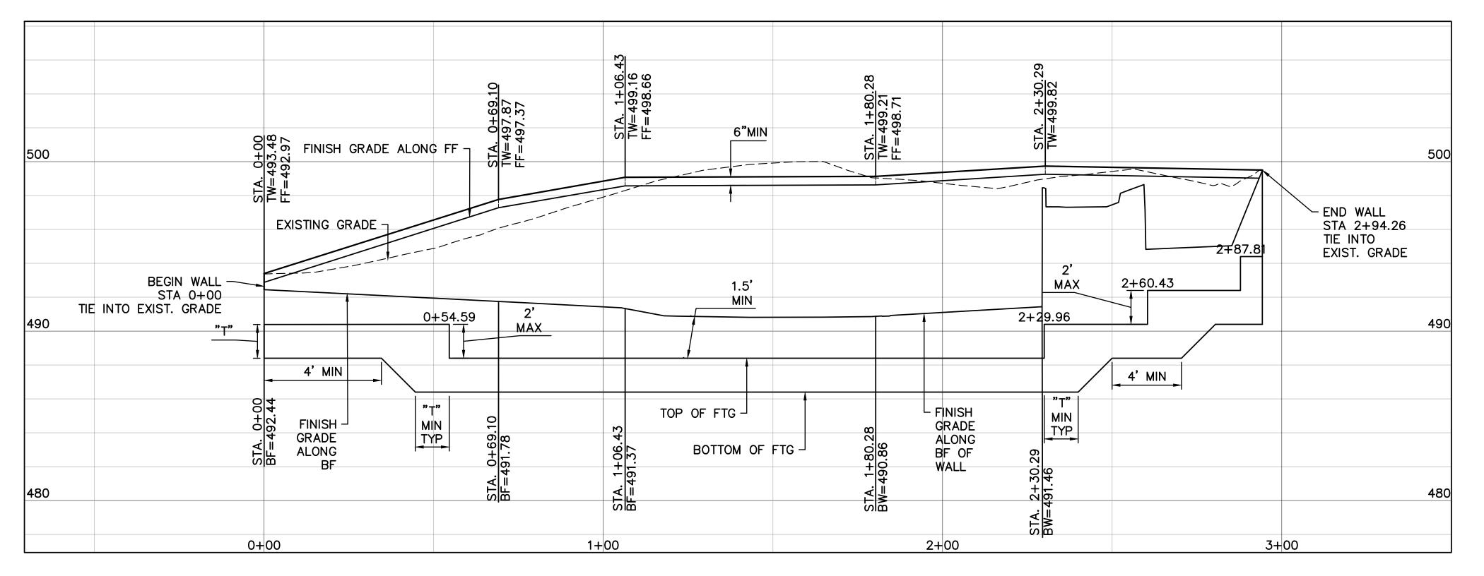
**LEGEND** NOTE: SEE PAGE 51, DETAIL 4 TOP OF WALL/BOTTOM OF WALL/FRONT FACE/ BOTTOM FACE FOR TYP WALL CORNER BEND DETAIL FTG FOOTING SCALE: 1" = 4' - 0"FOR TYP STEP FOOTING DETAIL SCALE: 1" = 20'-0"SEE RETAINING WALL SHEETS 55 & 56 FOR RETAINING WALL DETAILS REVISION DATE MADE BY APPROVED DESCRIPTION
