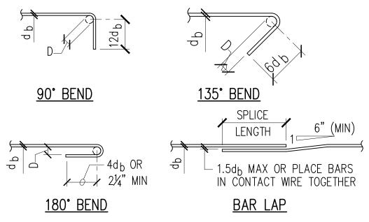
1. LENGTHS ARE FOR CONCRETE WITH REBAR SPACED AT 6 BAR DIAMETERS MINIMUM. INCREASE LENGTH BY 25% FOR BARS SPACED LESS THAN 6 BAR DIAMETERS 2. "TOP BARS" ARE HORIZONTAL BARS WITH
