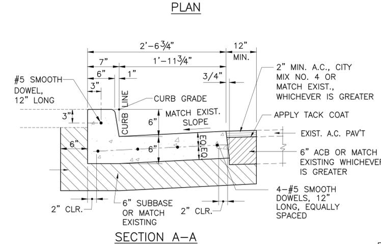
**EXIST. CURB AND GUTTER TO NEW CURB AND GUTTER CONNECTION DETAIL**
