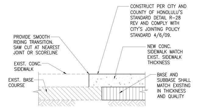
**CONCRETE SIDEWALK CONNECTION DETAIL**
