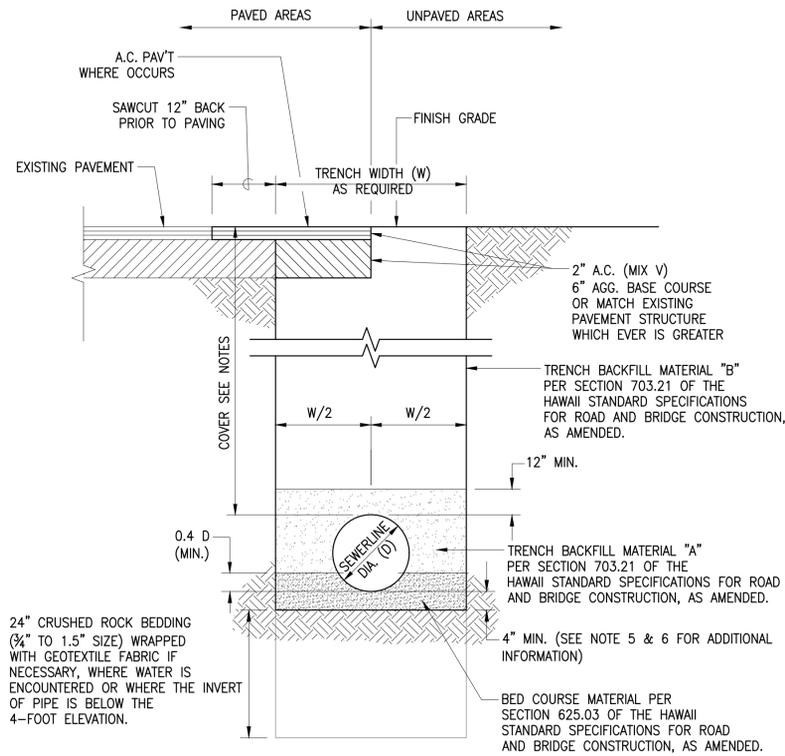
**TYPICAL TRENCH RESTORATION DETAIL FOR SEWERLINE**
