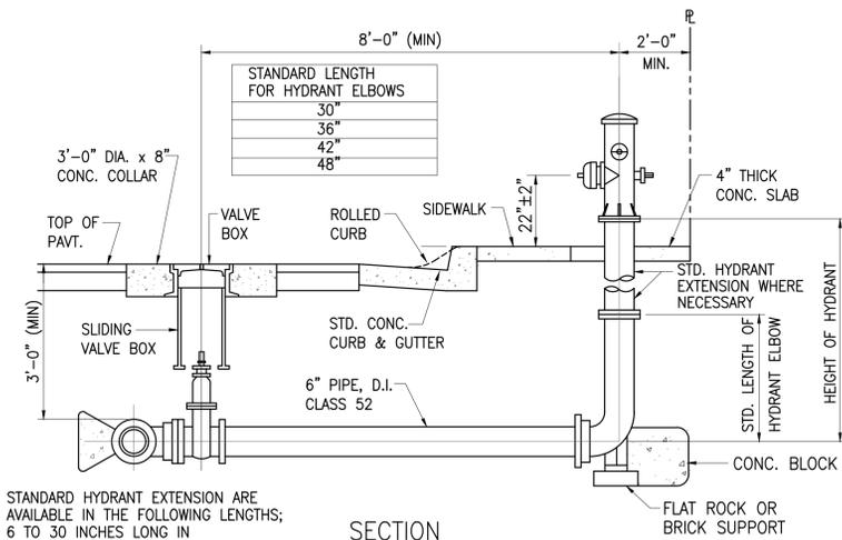
STANDARD HYDRANT EXTENSION ARE AVAILABLE IN THE FOLLOWING LENGTHS; 6 TO 30 INCHES LONG IN INCREMENTS OF 6 INCHES.
